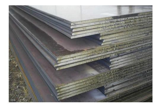
General specification: Thickness: 1.60mm - 6.0mm Width: Upto 1600mm Length: As per requirement Usage Automobiles, White goods, Roll forming, General Engineering & Fabrication, Packaging, Drum & Barrels, furniture etc.
